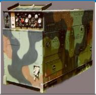
30 kW TQG Weight = 3005 lb. = 80' x 36" x 55" LxWxH 3ph, 4-wire Output = 120/208V = 240/416V = 50/60 Hz Fuel Use= 2.43 gph rated Fuel Tank= 23 gal Efficiency Curve 35 30 25 20 20 15 15 10 5 20 60 sò 40 100 n Output (%)
