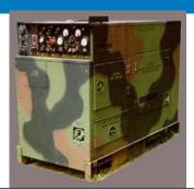
15 kW TQG Weight = 2124 lb. = 70' x 36" x 55" LxWxH 3ph, 4-wire Output = 120/208V = 240/416V = 50/60 Hz Fuel Use= 1.5 gph rated Fuel Tank= 14 gal Efficiency Curve 30 25 20 · 15 · 10 · 10 5 Ω. 20 40 60 sò 100
