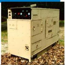
60 kW TQG Weight = 4063 lb. LxWxH = 87' x 36" x 59" 3ph, 4-wire Output = 120/208V = 240/416V = 50/60 Hz Fuel Use= 4.51 gph rated Fuel Tank= 43 gal Efficiency Curve 35 30 25
