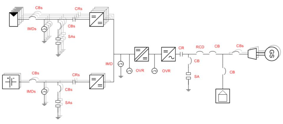
CB: Circuit Breaker IMD: Insulation Monitoring Device SPD: Surge Protection Device OVR: Over Voltage Relay RCD: Residual Current Device CR: Contactor
