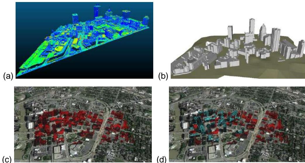
**Figure 1. Demonstration of image processing capabilities to extract individual building characteristics from point cloud data such as LiDAR: (a) data points from aerial LiDAR survey of downtown Rochester, NY, (b) resulting watertight building models, (c) rendering in Google Earth, and (d) ability to select individual buildings based on their geometric characteristics such as elevation. (Courtesy A. Lang)**
