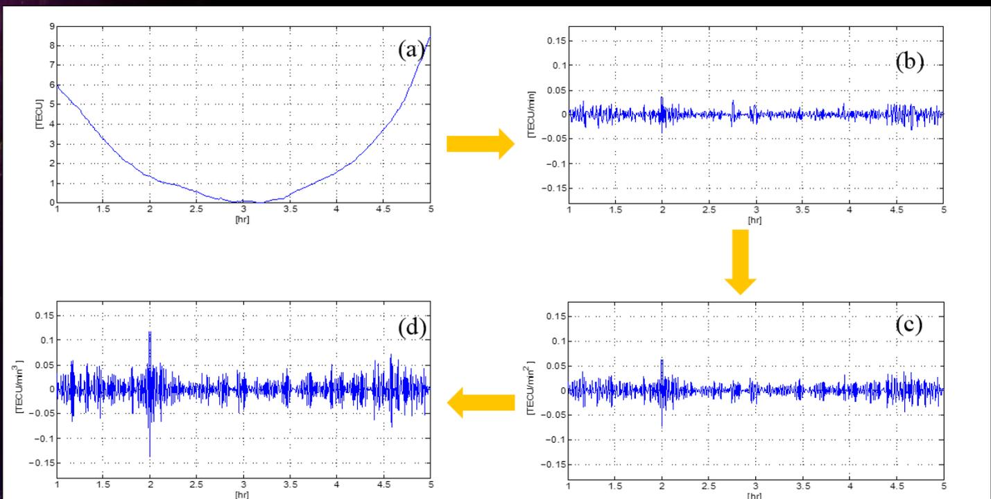
Figure 1: Numerical derivatives of STEC data span; (a) STEC, (b) the first order derivatives of STEC, (c) the second order derivatives of STEC, (d) the third order derivatives of STEC. (Released)
