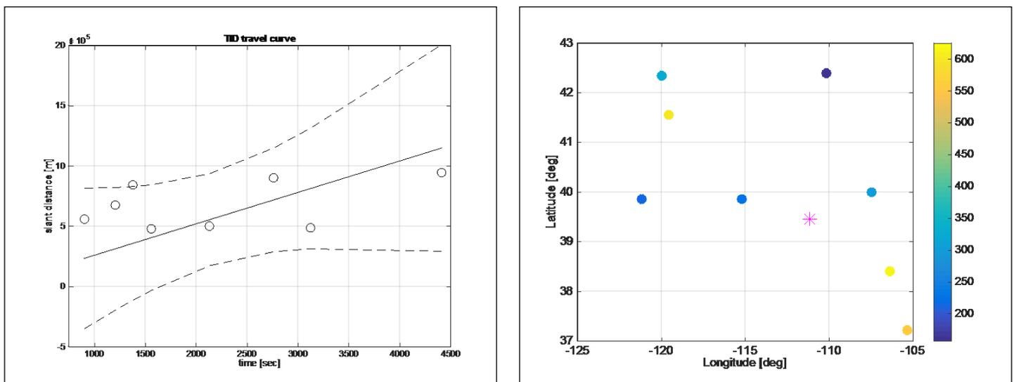
**Figure 4: TID velocity propagated from the 2007 Crandall Canyon Mine collapse; travel time curve with the 99 percent confidence interval (left) and TIDs at their ionospheric pierce points (right) where the color of each dot represents its travel velocity in m/s from the color bar. The pink star indicates the location of mine collapse. (Released)**
