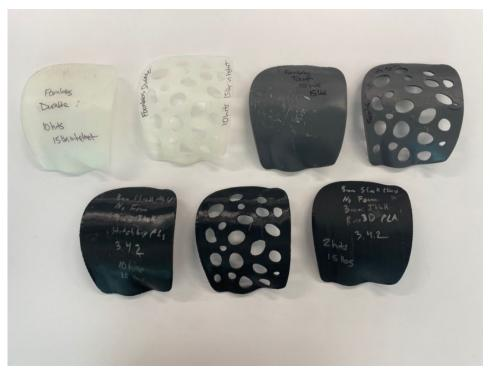
Figure #. Testing Guards (Top Row L-R: Formlabs<sup>®</sup> Durable resin, solid; Formlabs<sup>®</sup> Durable resin, holed; Formlabs<sup>®</sup> Tough resin, solid; Formlabs<sup>®</sup> Tough resin, holed; Bottom Row L-R: Hatchbox<sup>®</sup> PLA, solid; Hatchbox<sup>®</sup> PLA, holed; Raise3D<sup>®</sup> PLA, solid)
