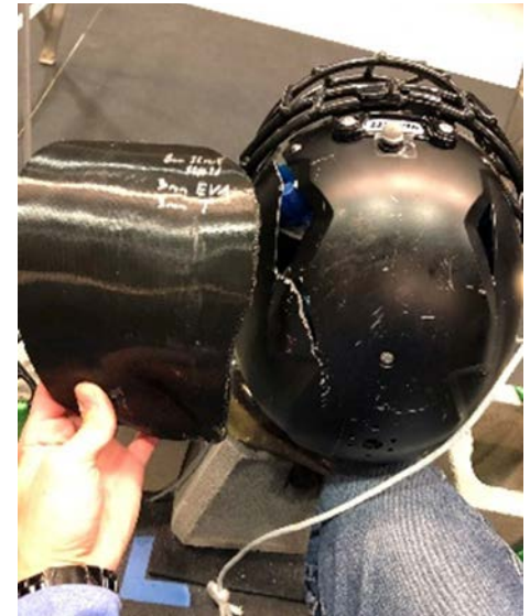
Figure 5. Final Impact of Helmet Weighted to 23.8 lbf Resulting in Fracture of Guard (Hatchbox PLA Solid) and Helmet (Source: M. Zabala and J. Larson).
