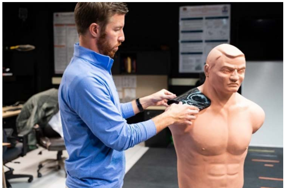
Figure 1. Custom-Fit, 3-D-Printed Shoulder Guards Fitting the BOB (Source: M. Zabala and J. Larson).
