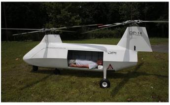
Figure 4-6. The DP-14 Designed to Carry 430-lb Useful Payload With a Large 23-ft<sup>3</sup> (Over 6 ft Long and 10 in Wide) Internal Cargo Area (Source: Dragonfly Pictures Inc. [78]).
