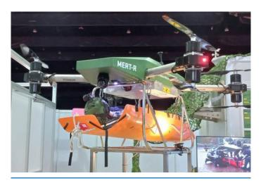
Figure 4-8. MERT-R MEDEVAC UAV Designed to Carry a Patient to a Medical Facility (*Source: Nondhasa* [86]).
