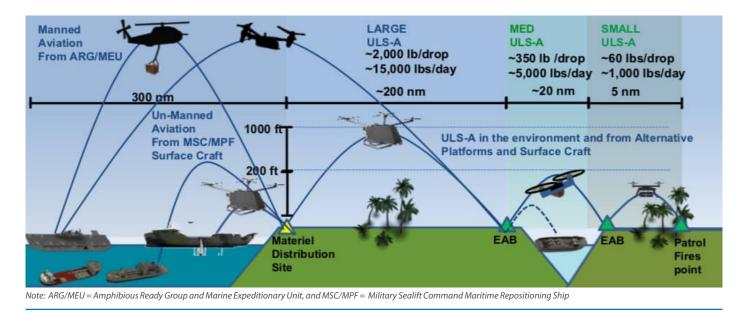
Figure 4-1. U.S. Marine Corps Graphic Showing How Small, Medium, and Large Unmanned Logistics Systems—Air (ULS-A) Could Provide Distribution Capabilities Within the Expeditionary Advanced Base Operations Environment in Conjunction With Conventional Aircraft (*Source: Head [64]*).
